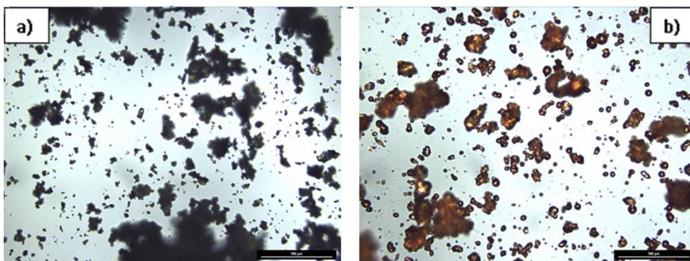
Fig-1: Optical micrographs of, a)TiC, b)Cu (200X) powders in as-received state
