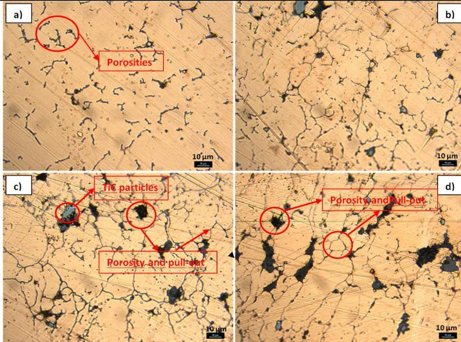
Fig-2: Optical micrograph images of, a) Cu, b) Cu-TiC (0,5wt%), c) Cu-TiC (1wt%), d) Cu-TiC(2wt%)
