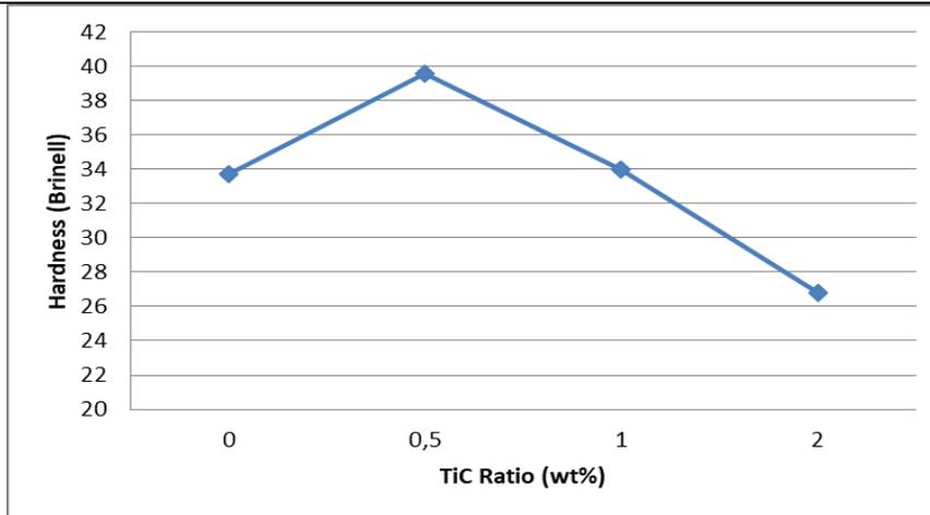
Fig-6: Change of the hardness with TiC content
