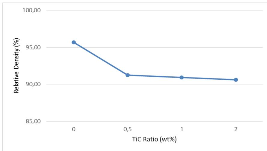
**Fig-5: Change of the relative density of specimens due to TiC content**
