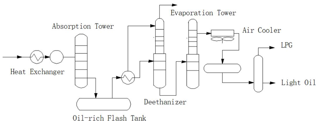
**Fig-3: Schematic diagram of the basic process of low temperature absorption**
