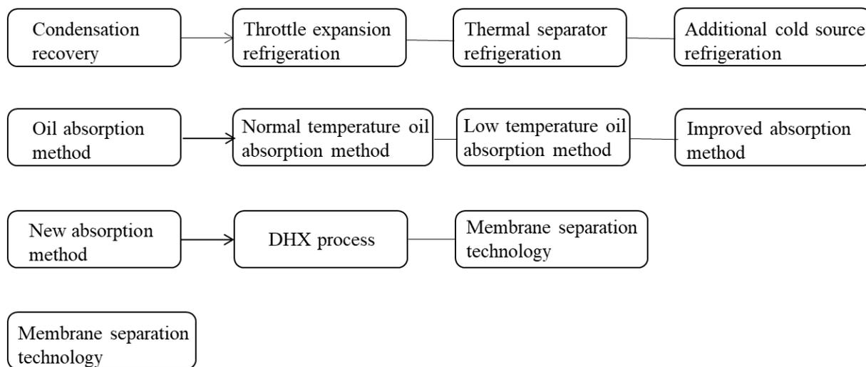
**Fig-2: Different light hydrocarbon recovery technology classification**
