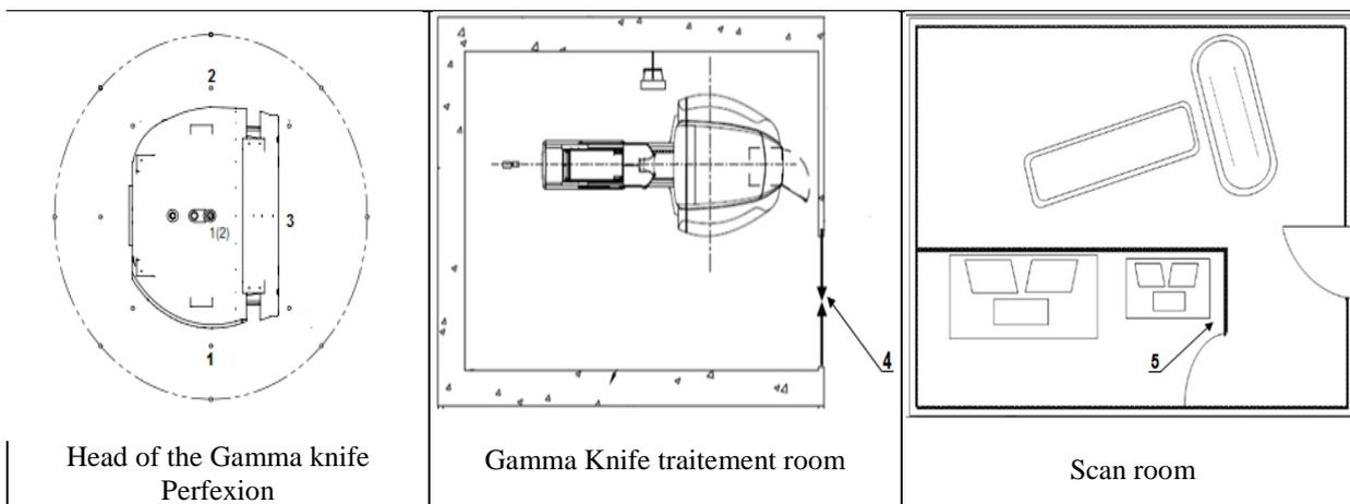
**Fig-1: Positions of measures taken by the Inspector detectors and RDS-31**
