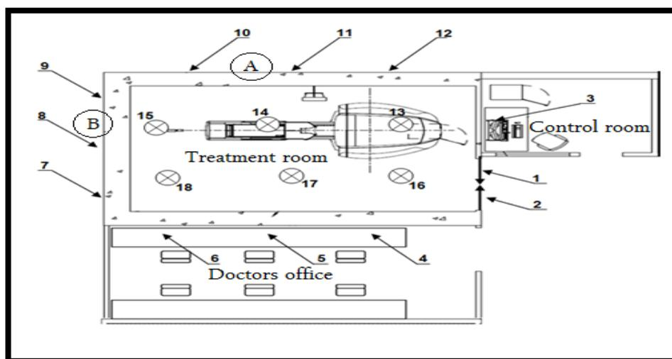
Fig-2: Positions of measures performed around the Gamma Knife treatment room
