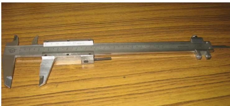
Fig-1: Vernier calipers of 0.2mms accuracy
