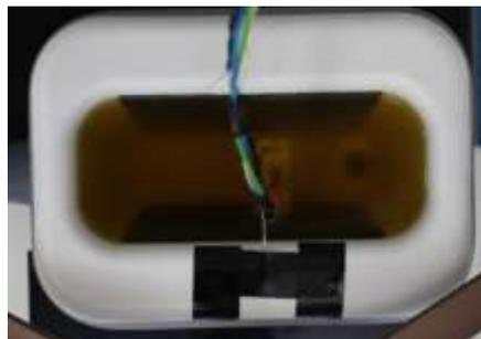
**Fig-9: Olive oil 70 minutes after starting the experiment. A change in transparency, obtained at a low temperature, is observed**
