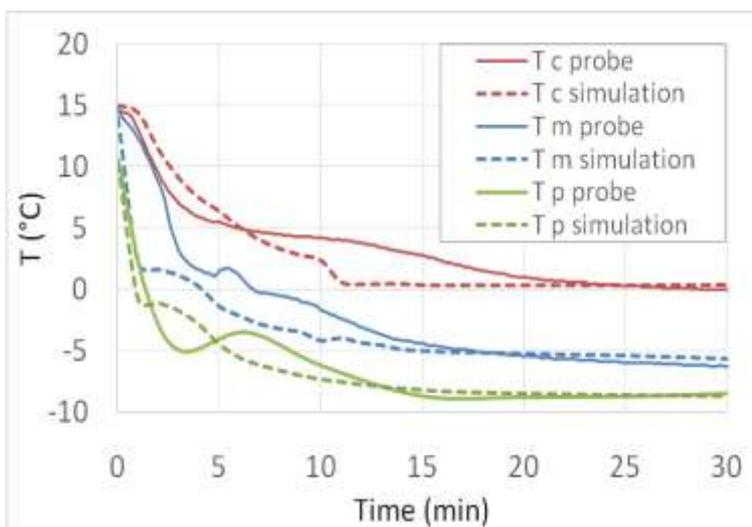
**Fig-4: Comparison of the water experiment (solid lines; Temperature values measured with probes) with the physical model (dotted lines; Temperature values simulated)**
