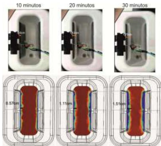
**Fig-5:** Comparison of the video frames of the water experiment with images from the simulation with ice formation at 10’, 20’ and 30’ after starting the Cooltech® process at -8 °C. The simulation images show the areas with phase changes in blue (ice) and without phase changes in red (water)
