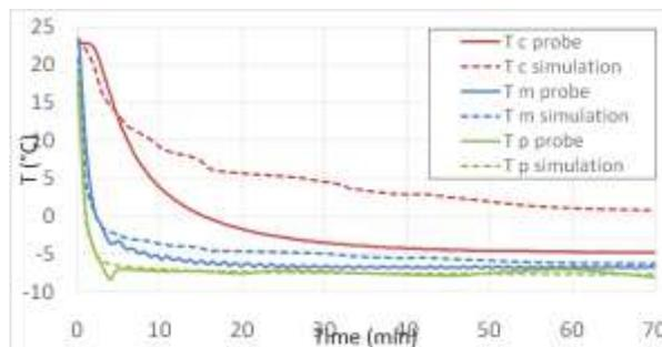
**Fig-8: Comparison of experimental data (solid line) and simulation of phase change adjusted to a phase-change temperature of 5 °C (dotted line)**
