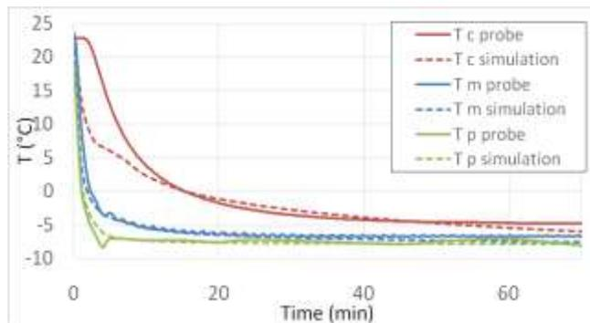
**Fig-10: Comparison of experimental data (solid line) and simulation of phase change adjusted to a phase-change temperature of -6 °C (dotted line) and latent heat of 80 kJ/kg**
