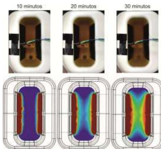
**Fig-11: Comparison of the video frames of the olive oil experiment at 10', 20' and 30' after starting the cryoadipolysis process with images from the simulation of viscosity, illustrated by a change of color from blue to yellow**
