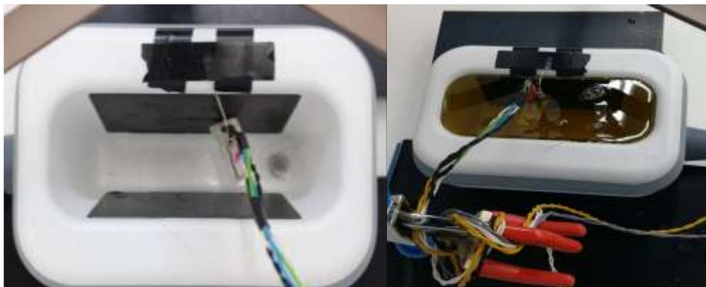
**Fig-1: Experimental set up. Cooltech® empty applicator, with temperature probes inside (above). Applicator with olive oil (below)**
