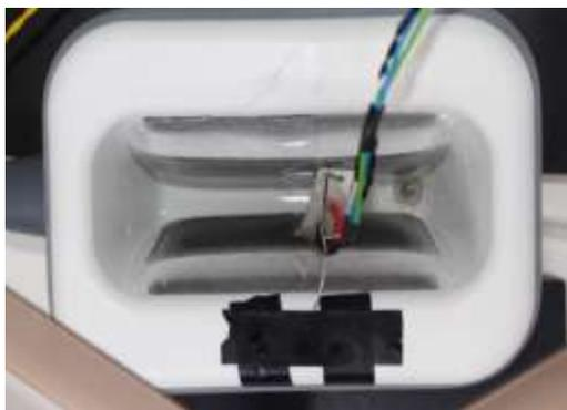
**Fig-6:** Frozen water in aluminum plates 30 minutes after starting the experiment.
