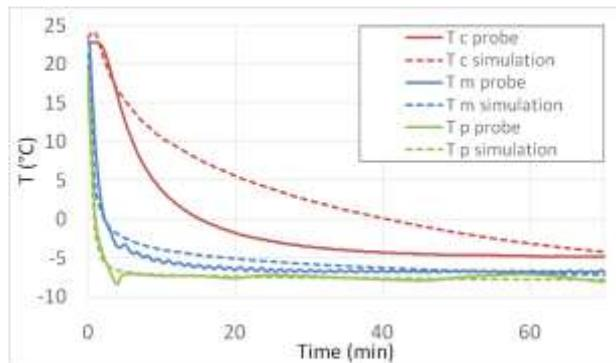
**Fig-7: Comparison of experimental data (solid line) and simulation without phase changes (dotted line).**
