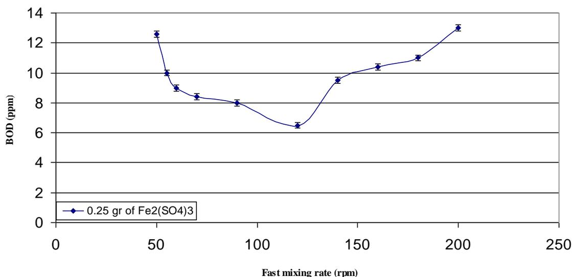
Fig 3: Value of BOD versus fast mixing rate
