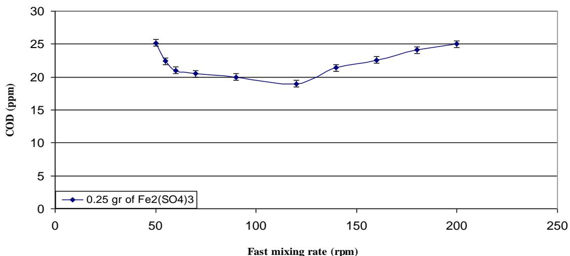
**Fig 2: Value of COD versus fast mixing rate.**
