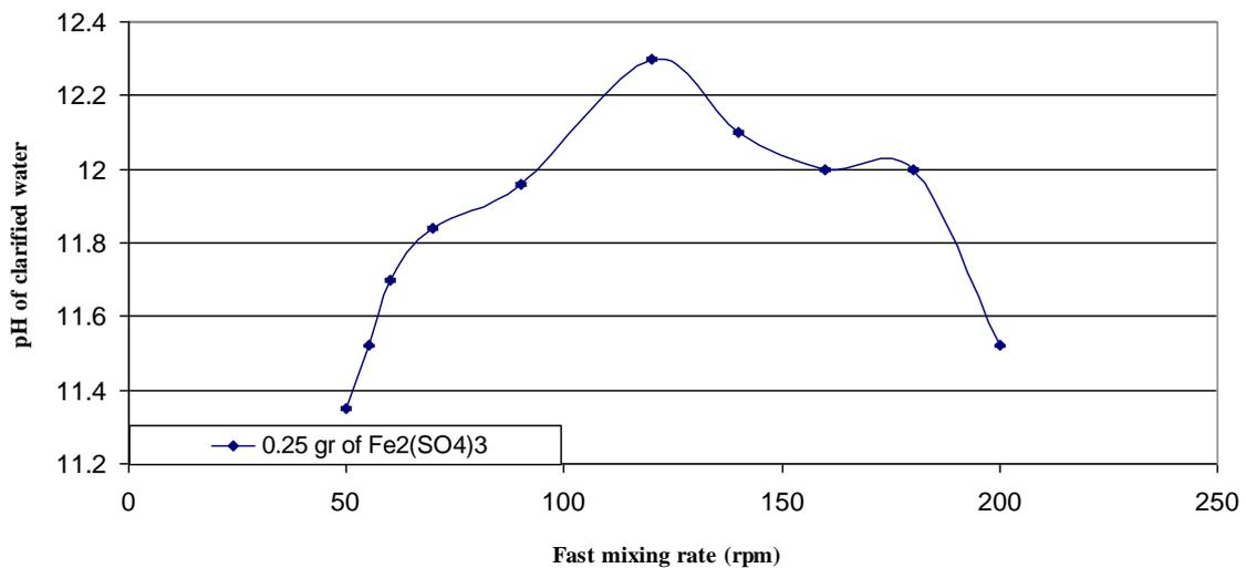
**Fig 1: Value of pH of clarified water versus fast mixing rate.**
