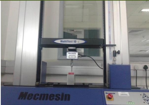
Figure 9: Fracture Resistance Test
