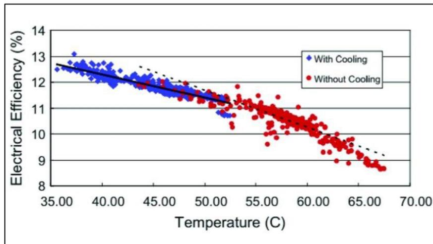
Figure 4: The relationship between solar cell efficiency and temperature (Adapted from Elsevier)
