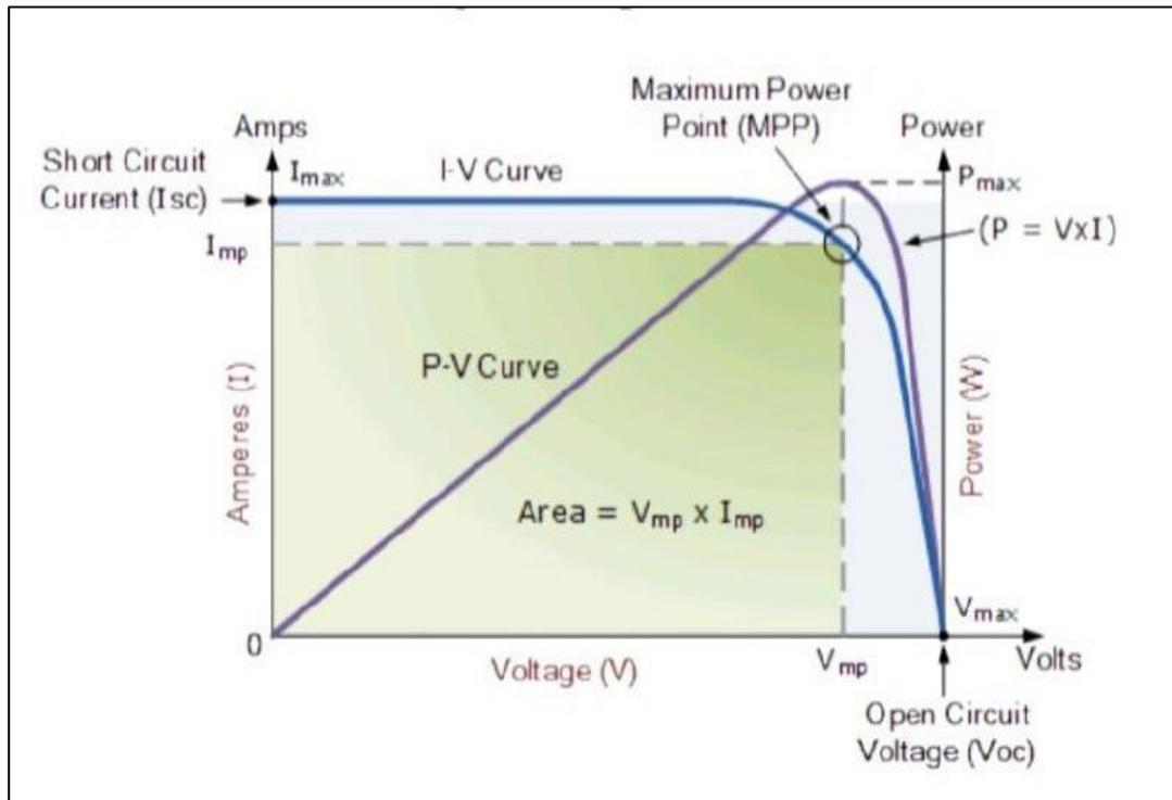
Figure 1: Solar cell I-V characteristic curves
