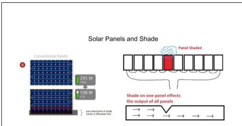
Figure 3: Shading effects on solar panel
