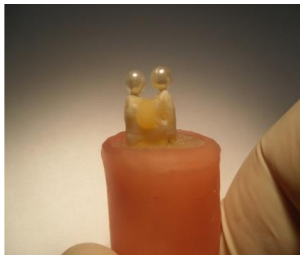
Figure 2: Specimen mounted in acrylic and reference balls cemented to cuspal tips
