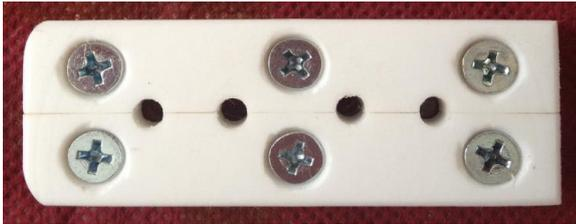
**Fig. 12: Teflon mold 4×6mm diameter used for sample preparation**
