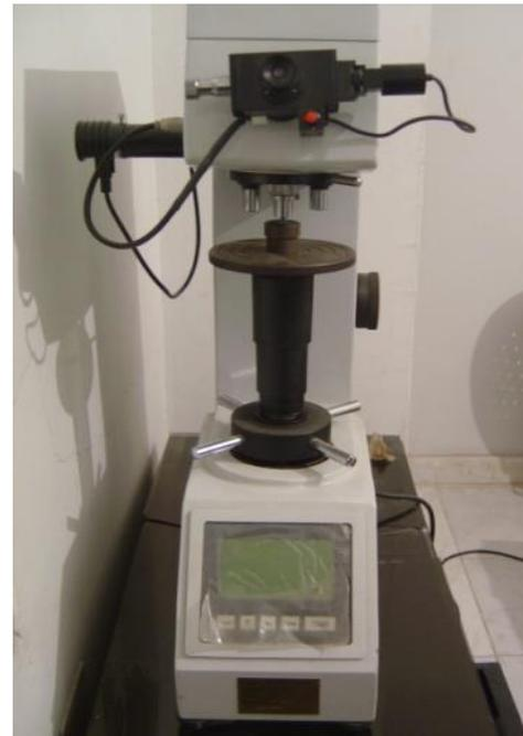
Fig. 11: Vickers Micro-hardness Tester
