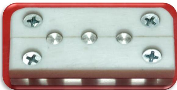
Fig. 9: Teflon mold 2×6mm diameter
