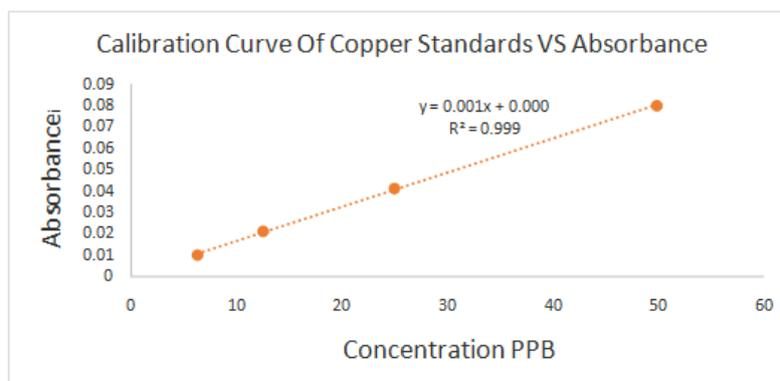
Fig. 1: Calibration curve, with different concentrations (PPB) been drawn to read unknown concentrations samples.
