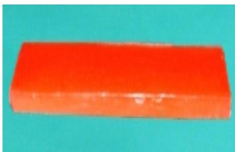
**Fig-2: Wax Specimen prepared using brass die**
