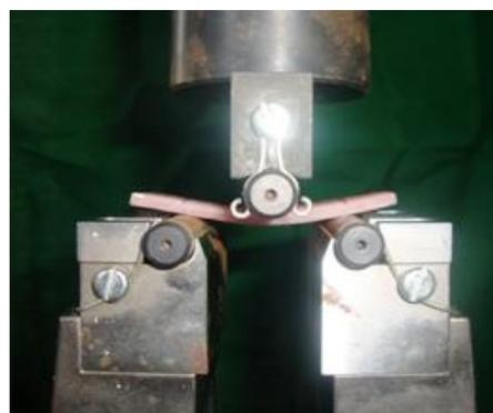
**Fig-6: Universal testing machine for three point bending test**
