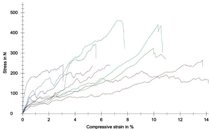
**Fig 2: Diagram recorded by an Instron machine. The amount of force required for a root fracture is shown by a sudden drop of force in the diagram.**
