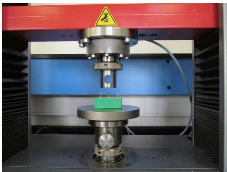
**Fig 1: Instron machine for inducing tooth fracture.**
