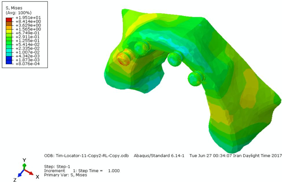
**Fig-3: Distribution of stress caused by the bilateral force in locator attachment-based overdenture**
