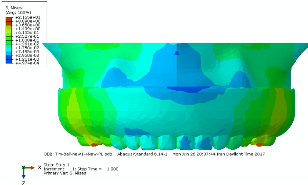
**Fig-1.** Distribution of stress caused by the bilateral force in ball attachment-based overdenture
