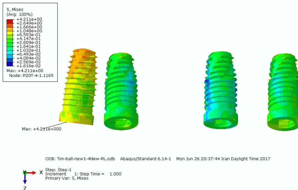
**Fig-2.** Distribution of stress caused by the bilateral force in ball attachment-based overdenture
