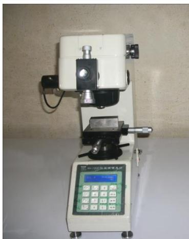
**Fig-1: Vicker's microhardness tester**
