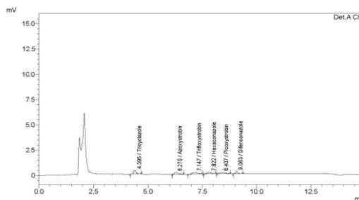
**Figure 1: Representative Chromatogram at fortification level of 0.03 µg/mL**
