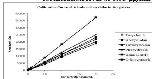
**Figure 2: Representative Calibration curve of triazole and strobilurin fungicides**
