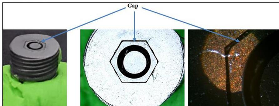
Cross section of an implant / abutment assembled at the hexagonal connection
