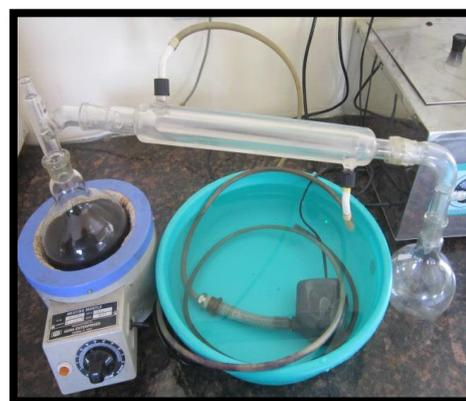
Fig-3: Distillation of the sample
