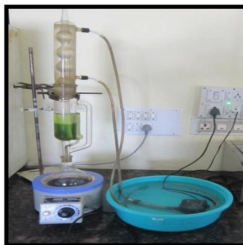
Fig-2: Soxhlet Apparatus extraction of the sample
