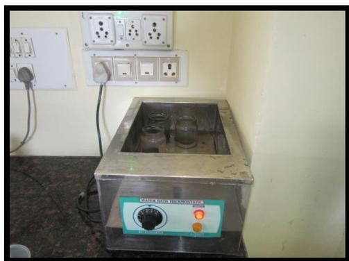
Fig-4: Drying of extract in water bath
