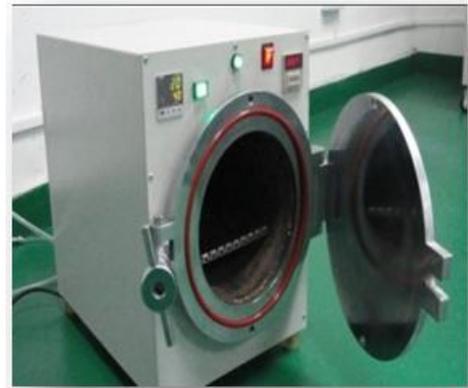
**Sterilization of Diluted Agar Medium in Autoclave**
